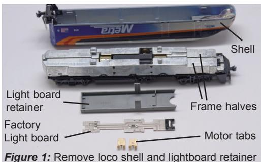
**Figure 1:** Remove loco shell and lightboard retainer
