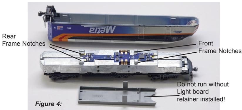
4. Install the DN163K4B decoder by tilting it slightly down at back as you insert the decoder into the rear frame notches. Carefully maneuver the decoder motor tabs down over the motor contacts and then level and slide the decoder board backwards so the board's corners are under the front
